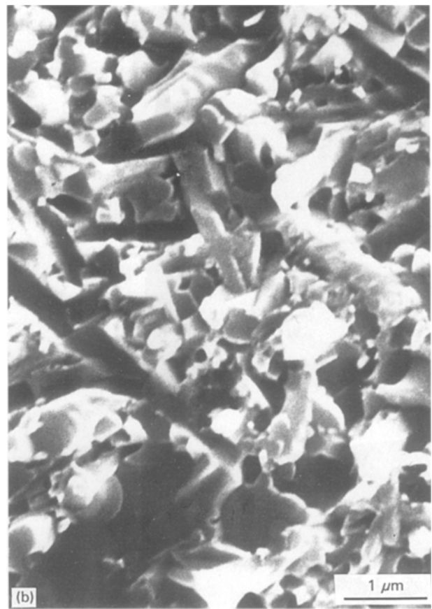
Figure 3 Microstructures of \text{Si}_3\text{N}_4 -celtsian materials: (a) M1A material, (b) material M1B and (c) material M1C.
